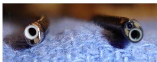
Figure 2: Comparison distal tip design X<sup>2</sup> (left) and X<sup>C</sup> (right)
