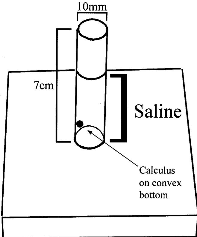
FIG. 2. In vitro caliceal model
